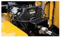
35 HP (26 kW) GAS ENGINE. The BC900xL is equipped with a Briggs & Stratton Vanguard gas engine, providing high torque in a compact and lightweight size to process branches and material up to 9" (22.9 cm) in diameter.
