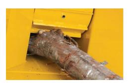
LARGE RECTANGULAR FEED OPENING. The large 9" x 14" (22.9 cm x 35.6 cm) feed opening helps boost productivity by reducing the need to trim heavily branched material before feeding it into the chipper.
