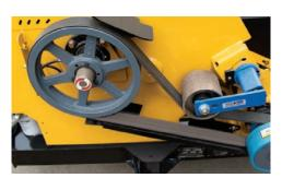
**CENTRIFUGAL CLUTCH.** The centrifugal clutch engagement prevents belt slip when engaging the clutch which means fewer maintenance costs.
